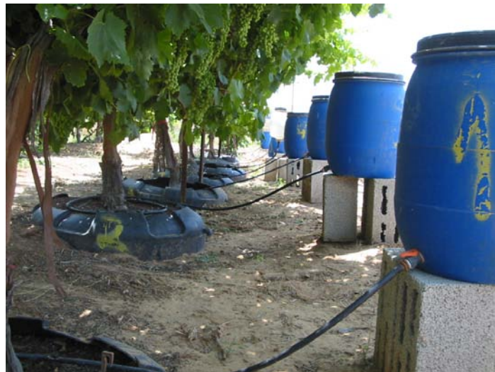
Figure 3. 80-L irrigation tanks (right) with the irrigation lines of each lysimeter (left).
