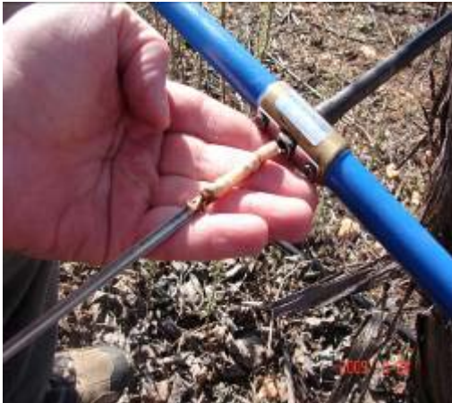
Figure 9. (left) Wood sampling using a 7-mm-diam. tree corer.
