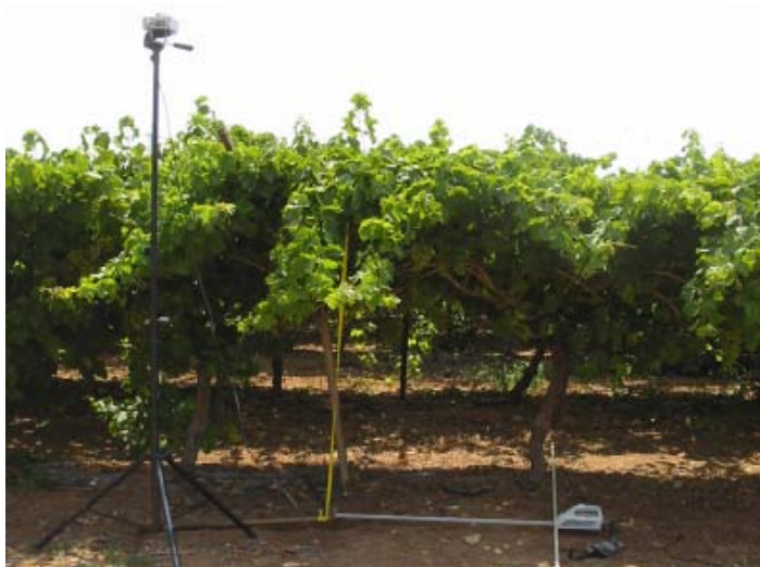
Figure 7. LAI measurement equipment. The beam fraction sensor (BFS) is located on top of the tripod (left). The line quantum sensor array and the data logger (Work about) is located beneath the vine canopy. A 20-cm graduated scale is located adjacent to the rows.
