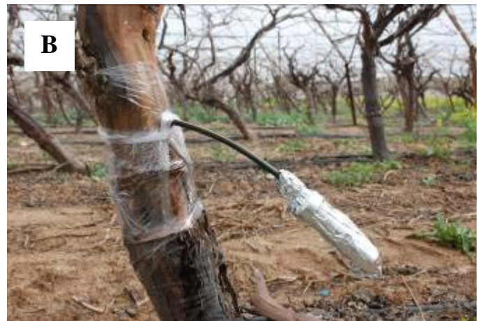
Figure 11. Xylem sap collection device. A. During installation. B. Tightly attached to the trunk and covered with aluminum foil after completion of installation.
