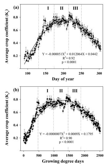
**Fig. 2.** (a) Development of crop coefficient ( $K_c$ ) as a function of day of year. (b) Development of crop coefficient ( $K_c$ ) as a function of growing degree days.Phenological stages (I, II, III) are marked by dashed lines. Each point is the mean of six lysimeters. Vertical bar denotes one standard error. Measured from 2012 to 2017 in a 'Cabernet Sauvignon' vineyard, Kida Israel.
