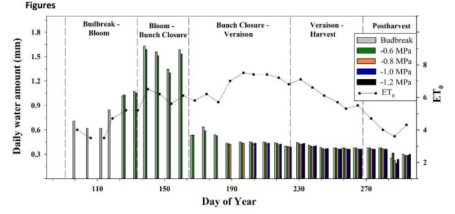
**Fig. 1** Seasonal pattern of water amounts applied to different irrigation treatments and ET<sub>o</sub>. Each bar represents one irrigation (once a week) expressed as daily water amount. Each treatment initiated to receive irrigation according to his threshold, then irrigated continuously until the end of growing season. 'Cabernet Sauvignon' vineyard 2016, Kida Israel.
