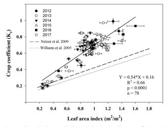
Fig. 4. Relationship between leaf area index (LAI) and crop coefficient ( $K_c$ ). Each point is the mean LAI of six vines, and the mean  $K_c$  of weekly water consumption of six lysimeters. Vertical and horizontal bars denote one standard error. Measured from 2012 to 2017 in a 'Cabernet Sauvignon' vineyard, Kida Israel.
