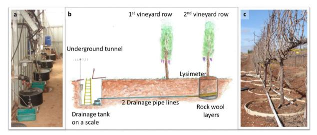
Fig. 1. General scheme of the lysimeter plot illustrating (a) drainage collection underground tunnel, the 30 l drainage collection tanks (black) mounted on scales in the underground tunnel; (b) a schematic side view of the system; and (c) an aboveground view of the six vines planted in the lysimeter tanks in the 2nd row of the vineyard.
