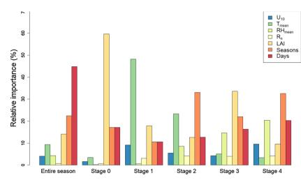
**Fig. 3.** Relative importance (%) of each variable on crop evapotranspiration for each phenological growth stage and for the entire season. The variables that were considered in the models were daily mean wind speed ( $U_{10}$ ), daily mean temperature ( $T_{mean}$ ), daily mean relative humidity ( $RH_{mean}$ ), total daily radiation (Rn), leaf area index (LAI), Seasons (between 2013 and 2017), and Days (183 per growing season). *Vitis vinifera* cv. 'Cabernet Sauvignon', Kida.2013–2017.
