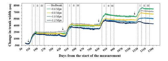
**Fig 4.** Multi seasonal (2014 - 2017) curve of the change in the trunk width of grapevines from different irrigation treatments. Budbreak at each year is marked by an arrow. Each line represents an average of 4 dendrometers. 'Cabernet Sauvignon' vineyard, Kida Israel.
