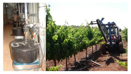
Fig. 1. The lysimeter system (a) Below-ground drainage collection tanks on scales; and (b) Vitis vinifera cv. 'Cabernet Sauvignon' vines planted in lysimeters during mechanical hedging. Kida Vineyard, 2014.
